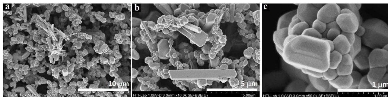
Figure 5. FESEM micrographs of the 1 h processed specimen after annealing at 700 °C for 90 min at different magnifications; (a,b) detachment of nanotubes and (c) formation of a coarse particle structure
